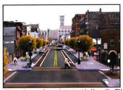
Above: Image of complete street in Knoxville, TN with similar dimensions to Broadway in Kingston. The roadway configuration incorporates wide sidewalks, clearly defined crosswalks, designated bike lanes and two travel lanes for motor vehicles.
