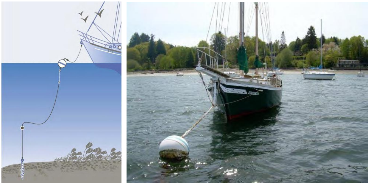
Figure 5: Typical Mooring section view and application
