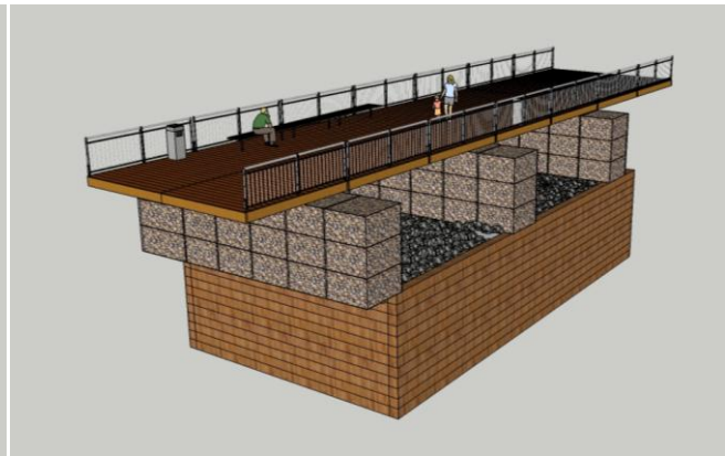
Figure 29 – Walkway, Option 3, with existing jetty
